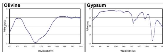
Figure 3: Example of prototype Ma-Miss instrument response signal taken in Olivine (volcanic rock) (left) and Gypsum (right). *Credit: INAF-IFSI*
