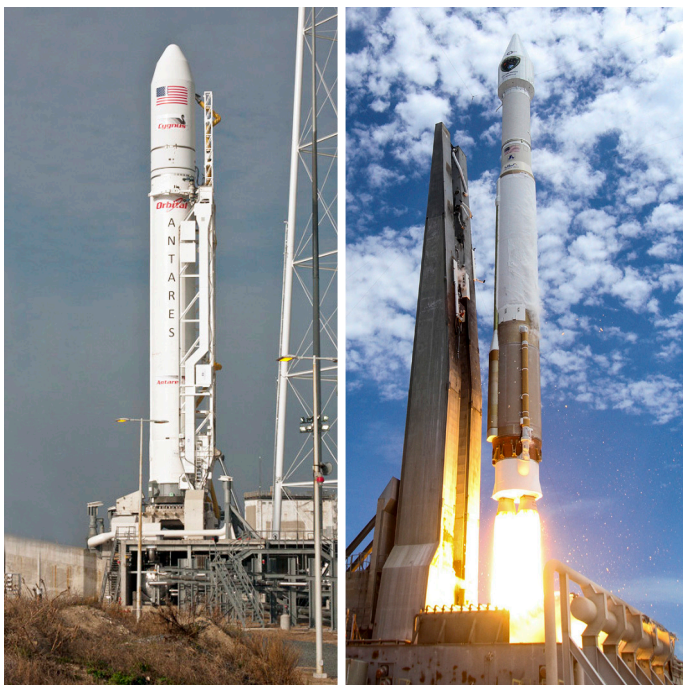
For CRS Missions, Cygnus is boosted into orbit by Orbital ATK's Antares™ medium-class space launch vehicle (left) or a United Launch Alliance Atlas V rocket (right)
